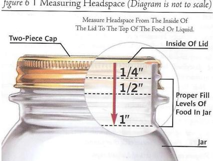
figure 6 | Measuring Headspace (Diagram is not to scale)
